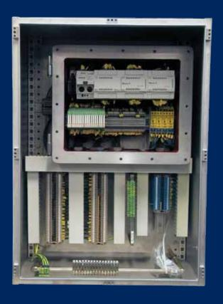
Tranberg enclosure system TEF1060 also includes solutions for encapsulating smaller EEx d enclosures for Non-Ex components. Our solution is to use an aluminium EEx d enclosure inside a TEF1060 EEx e Stainless Steel 316L cabinet. This results in a very flexible and cost efficient solution.
